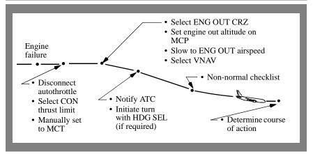
**Note:** If the airplane is at or below maximum ENG OUT altitude when an engine becomes inoperative, select and execute the ENG OUT CRZ page. Maintain engine out cruise speed using manual thrust adjustments.
