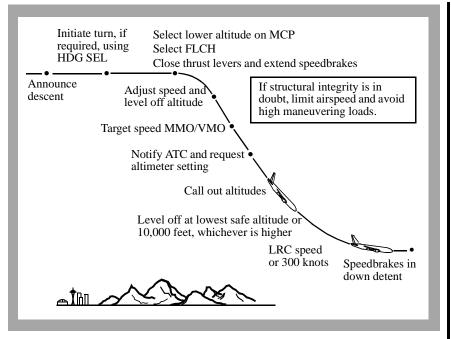
If the descent is performed because of a rapid loss of cabin pressure, crewmembers should place oxygen masks on and establish communication at the first indication of a loss of cabin pressurization. Verify cabin pressure is uncontrollable, and if so begin descent. If structural damage exists or is suspected, limit airspeed to current speed or less. Avoid high maneuvering loads. Maneuvers
