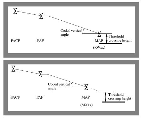
**Note:** The final approach course fix (FACF) is typically located on the final approach course approximately 7 NM before the FAF. The FAF referred to in the following procedures refers to the charted FAF and is intended to mean the point at which the final approach descent is begun.
